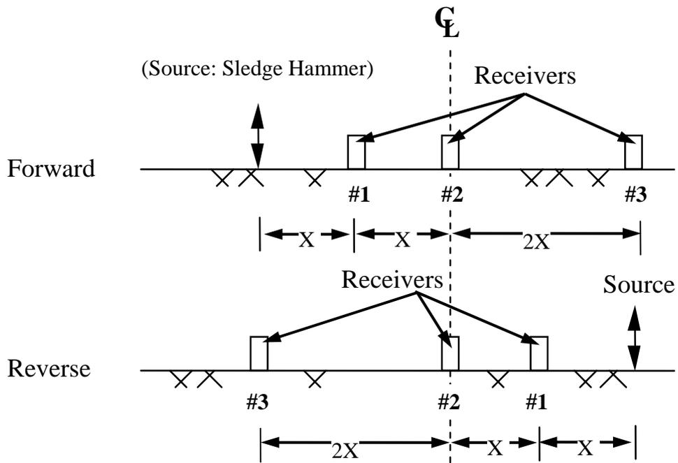
Figure 3 Common-Middle-Receiver Geometry Used in SASW Testing at Hanford Sites
