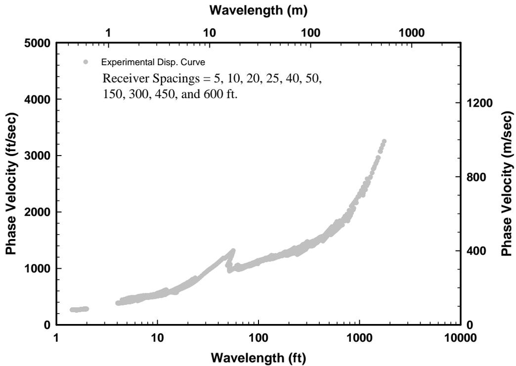
Figure 11 Composite Experimental Dispersion Curve Created from Phase Measurements Performed at all Receiver Spacings at Site H1
