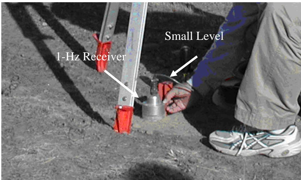
Figure 4 Photograph of 1-Hz Geophone Semi-embedded in the Ground and the Pre-test Check for Plumbness
