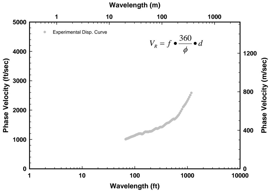
Figure 10 Individual Dispersion Curve Created from the Unwrapped Phase Record in Figure 12a Measured with a 600-ft Receiver Spacing at Site H1
