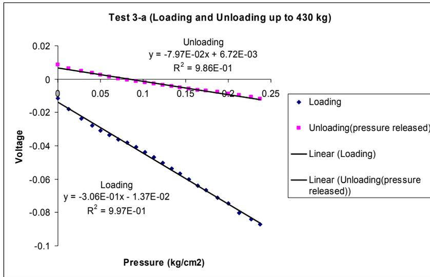
**3-b:** Loading and Unloading up to 430 kg with released pressure.
