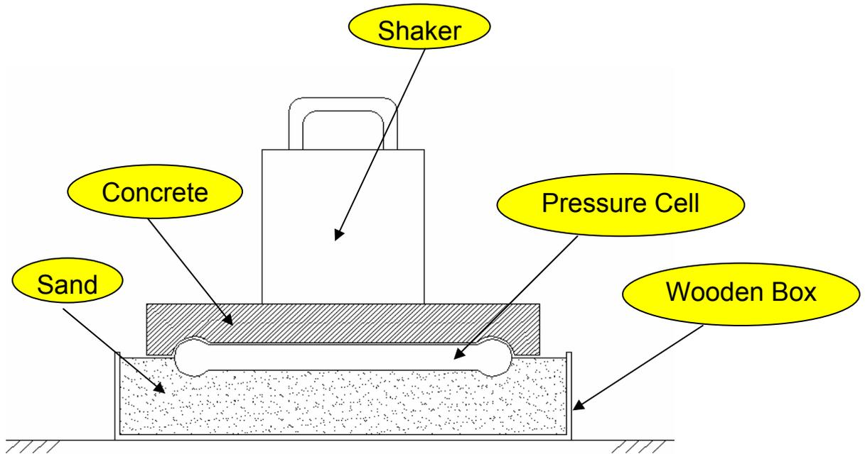
Schema of Dynamic Calibration Test Setup
