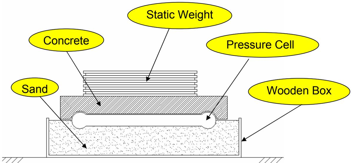
Schema of Static Calibration Test Setup
