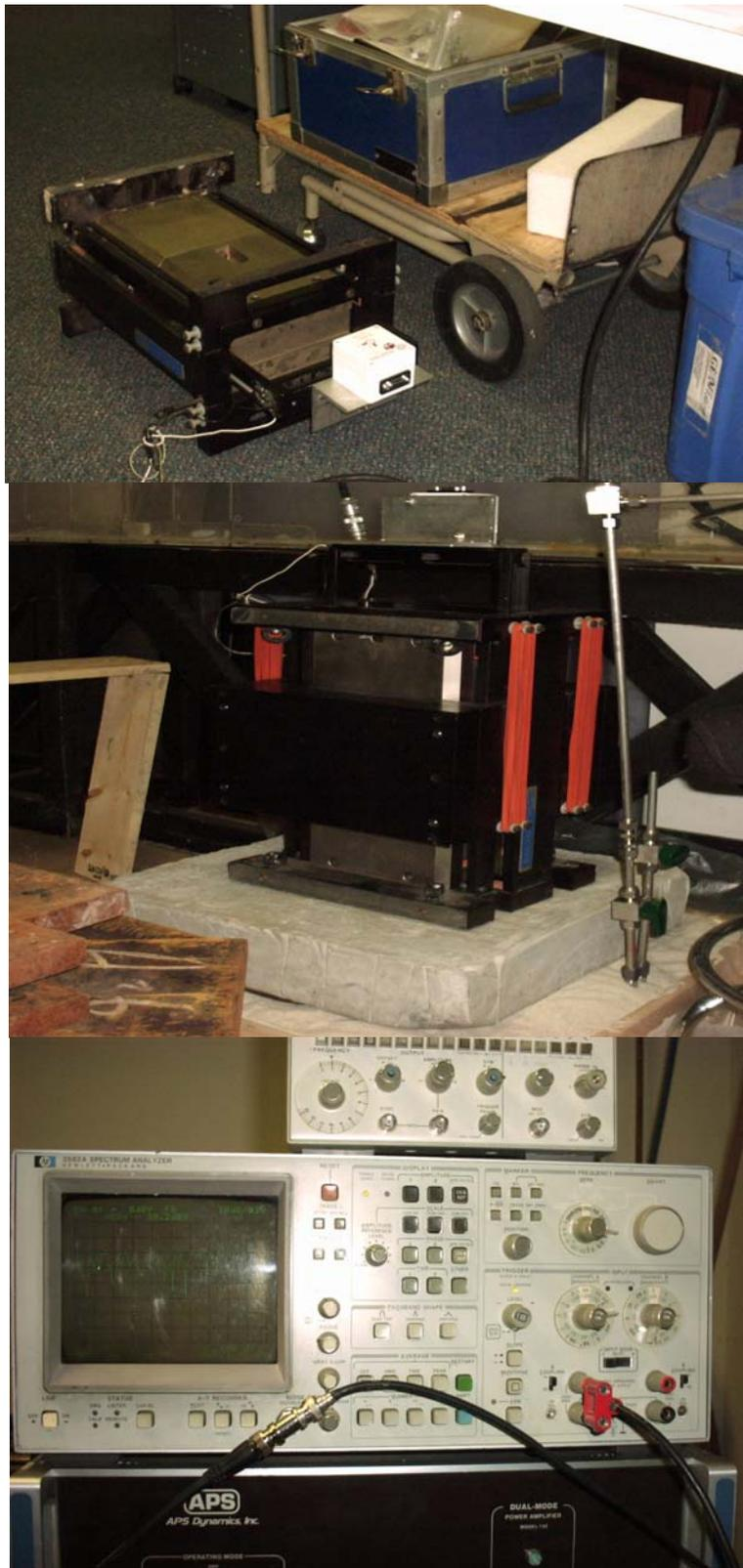
Shaker setup, dynamic calibration and spectrum analysis system
