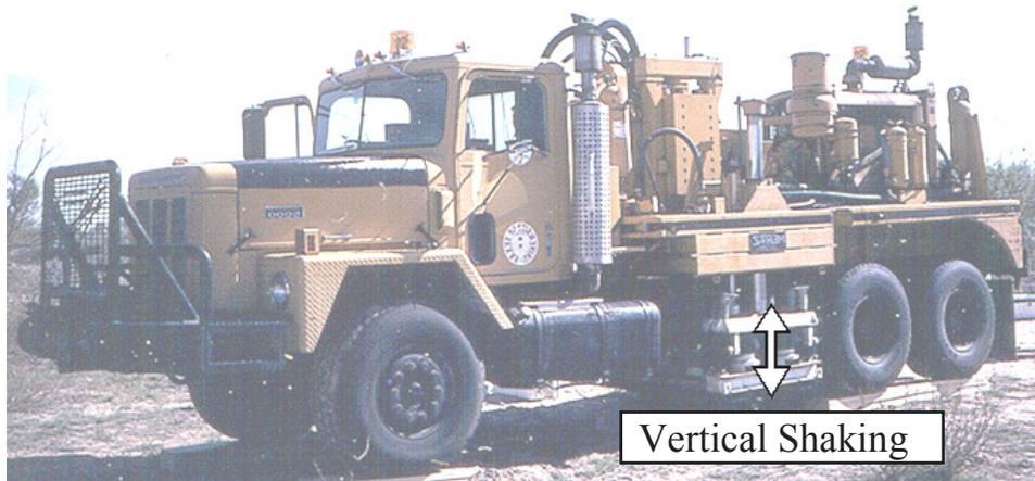
Figure 3-1 Picture of the vibroseis truck used as a dynamic source in the first-generation in-situ liquefaction tests (from Stokoe et al., 2004).
