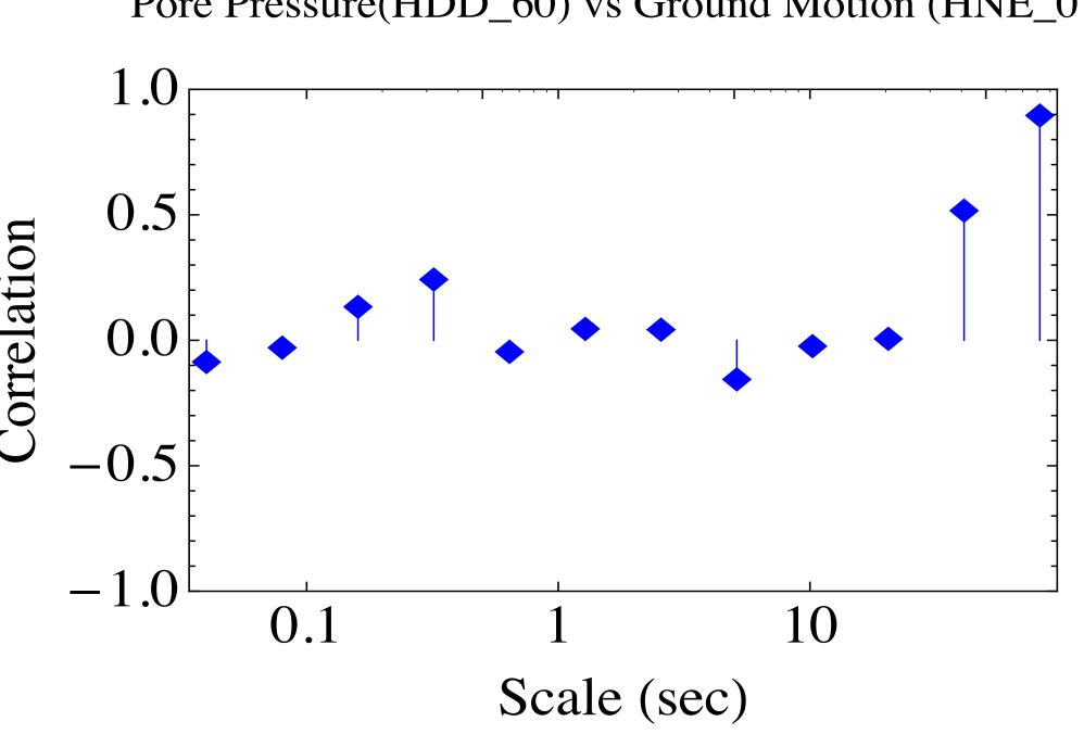
Figure 9: Correlation of the pore pressure signal with the East component of ground acceleration computed for scale values in Figure 8. At long-period scales, the pore pressure signal correlates well with the ground motion.
