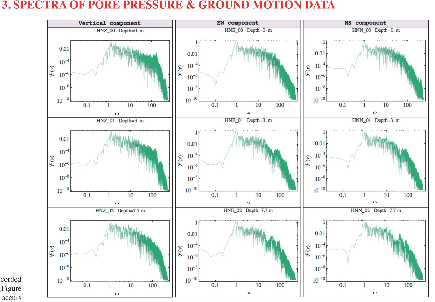
Figure 6: Angualr frequency spectra of the three components of ground motion computed for a time window of 300 sec (Figure 4). The shapes of the curves are complicated, especially for the EW and NS components, and there is no simple functional representation. Note that for the EW and NS components at 3 m and 7.7 m depths, there are depletions of the spectral curves at several angular frequencies in the range 10 to 100 rps.
