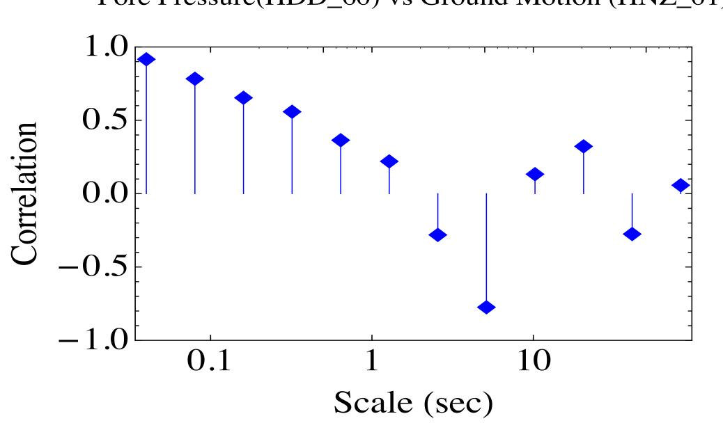
Figure 10: Correlation of the pore pressure signal with the Vertical component of ground acceleration computed for scale values in Figure 8. Note the high correlation with small scales in seconds (relatively higher frequencies).
