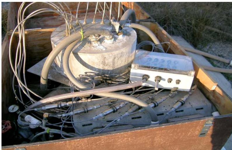
Each sensor is wired into the Lightning Protection box and then back to the hut in a multi-pair cable.
