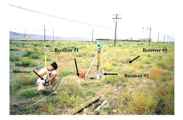
Figure 5 Photograph of Mr. Min Jae Jung Using the Sledge Hammer Source at Hanford Site H9
