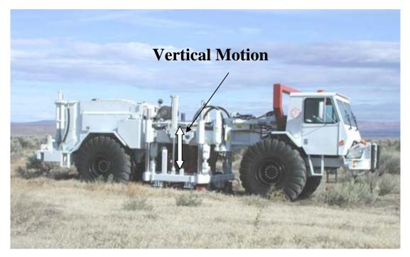
Figure 6 Photograph of Liquidator Operating in Stepped-Sine Mode at the Hanford Site H10
