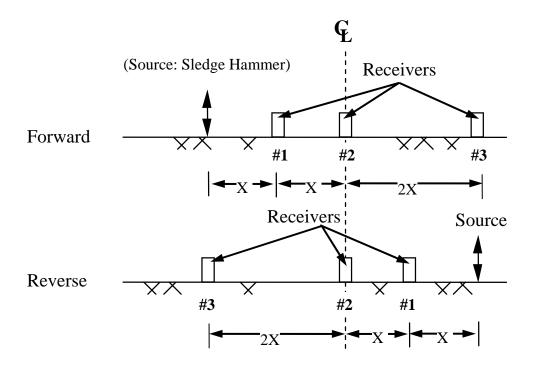
Figure 3 Common-Middle-Receiver Geometry Used in SASW Testing at Hanford Sites
