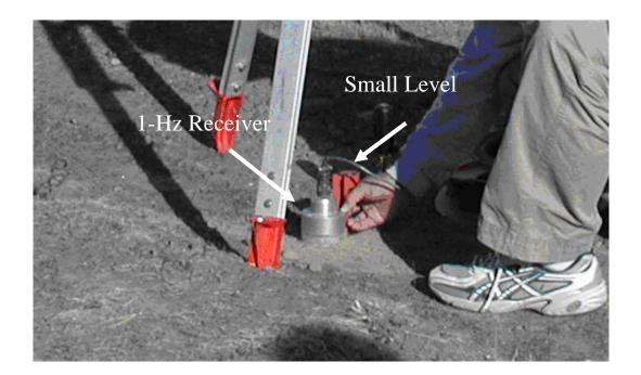
Figure 4 Photograph of 1-Hz Geophone Semi-embedded in the Ground and the Pre-test Check for Plumbness
