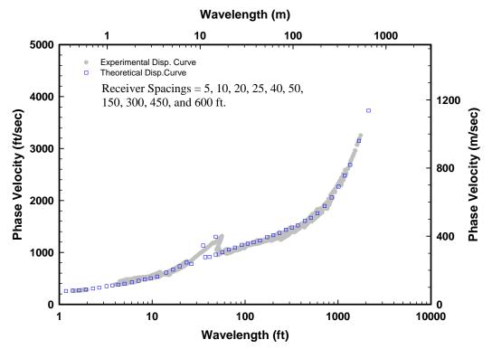
Figure 13 Comparison of the Fit of the Theoretical Dispersion Curve to the Experimental Dispersion Curve at Site H1
