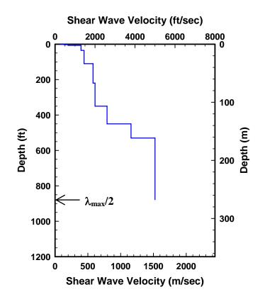
Figure 14 Final Shear Wave Velocity Profile Determined at Site H1
