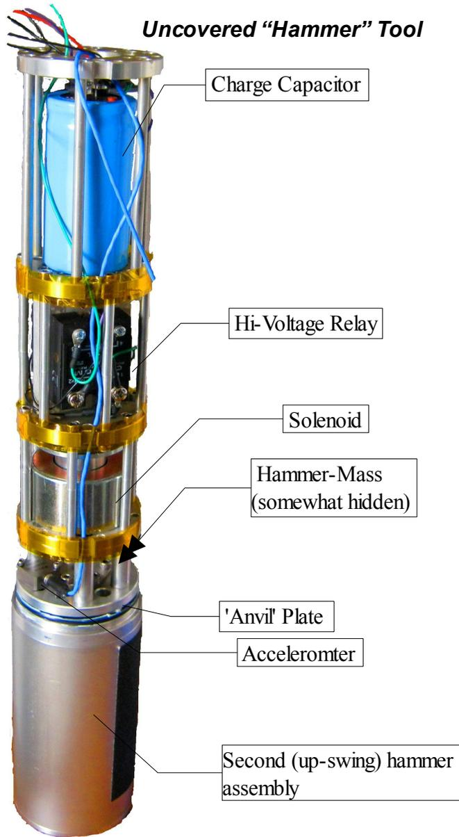
Working from a 12V supply, a high-voltage up-converter DC-DC converter (at the wellhead, not part of the downhole tool) charges the Capacitor.
