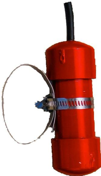
The Geophones are passive velocity sensors. The sensors used are Geospace GS-20DX 14 hz, They are set for 70% damping.
