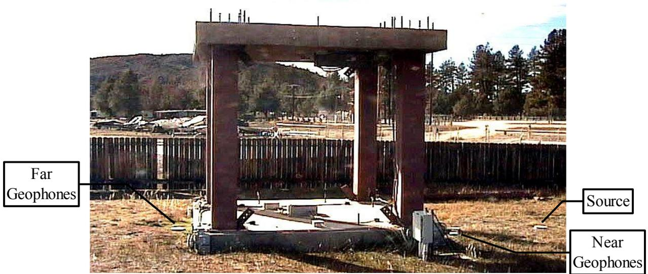
The cabling from the 'hammer' and the geophones is brought from the top of the boreholes to the metal junction box at the front-right corner of SFSI structure and from there into the instrumentation-hut via underground conduit entering the hut through the stainless steel trough-box on the side of the building. Inside the hut the cables connect to the hammer-controller circuit board and to the Kinometrics Granite Data-Acquisition system.
