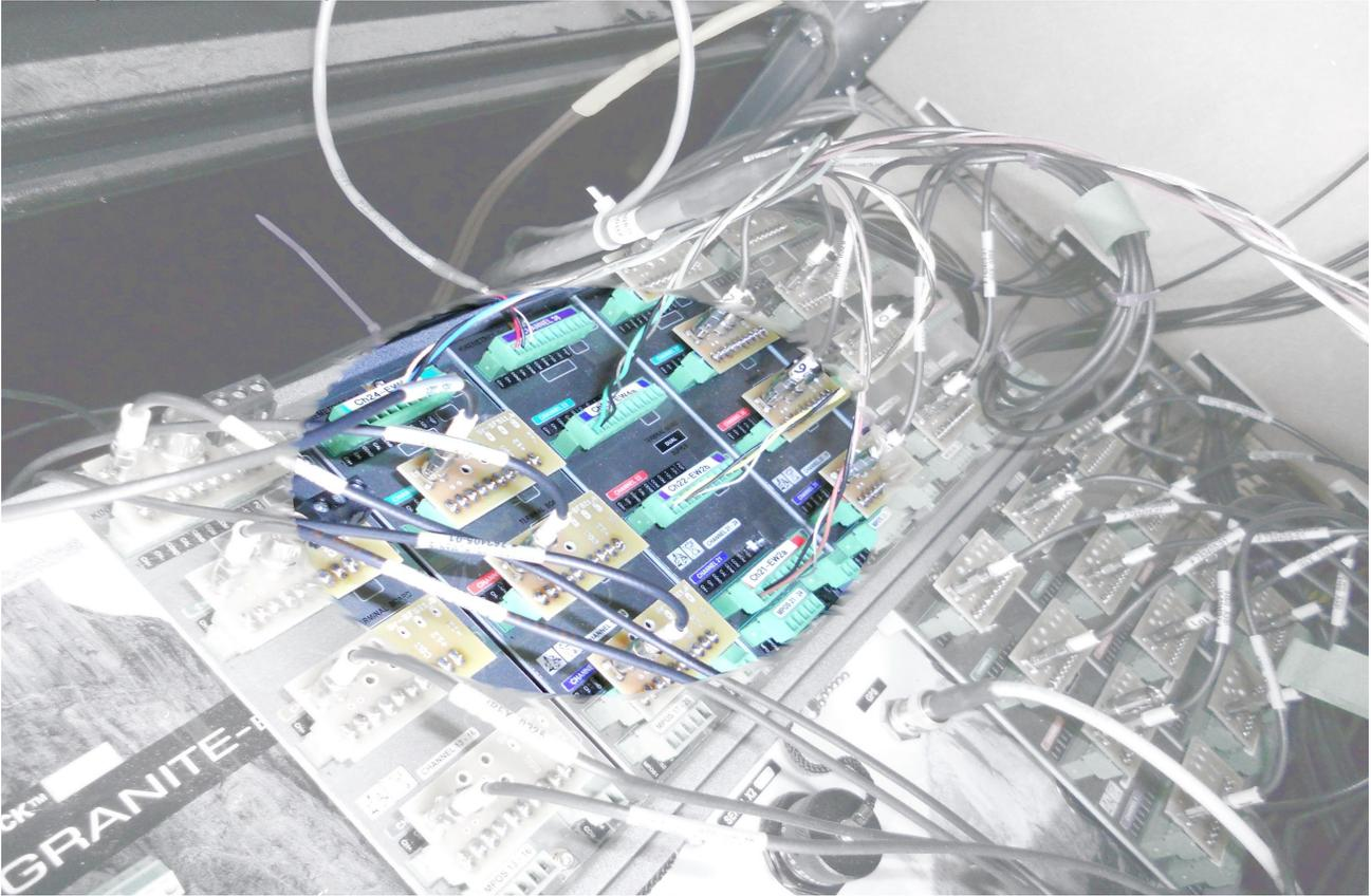
The Granite is configured with 40 virtual channels made up of the 36 physical channels sampled continuously at 200sps and four of the Velocity measurement channels (21-24) additionally sampled at 2ksps on an sta/lta triggered even basis.
