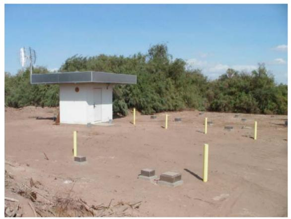
Figure 3. Photo of WLA with instrument hut and stainless steel boxes over instrument casings
