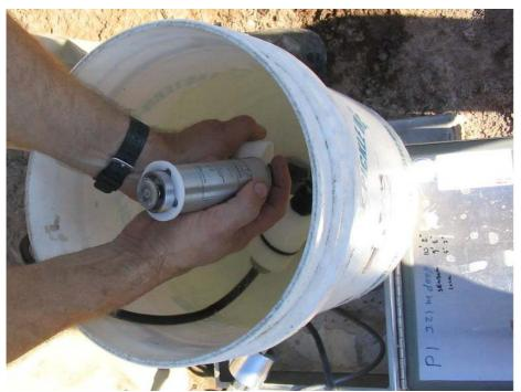
Figure 9. Pressure transducer, sensing element upward without filter, being saturated in bucket of water in preparation for installing the assembly in casing below the bucket
